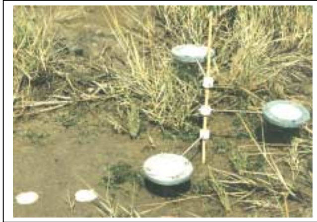
Figure 1. Determination of the rate of sedimentation during a single tide at Waarde marsh, in the Westerschelde. The weight of sediment deposited on the papers on the mud surface were close to that measured when the paper holders when used at that level.
